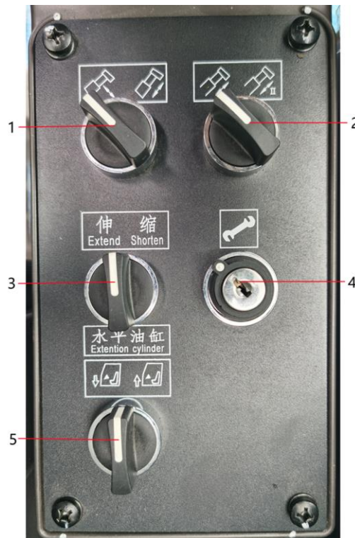
Figure 4-38 Position of switch for controlling crawler carrier extension and retraction
